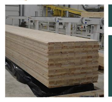
VAARA Stabil<sup>™</sup> NON SETTLING CLT-LOGS ARE AVAILABLE EITHER NON-PROFILED OR READY PROFILED 12-METER LONG, WITH PINE OR SPRUCE SURFACE ACCORDING TO CHOICE.
